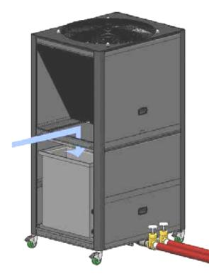
• If the optional automatic water makeup system was not installed on the chiller, remove the side panel to the left of the process connections and fill the tank and chilled water circuit piping until the tank is approximately <sup>3</sup>/<sub>4</sub> full. Fill with water (or a water/glycol mixture if the desired setpoint is lower than 45°F (7°C)). The water/ glycol mixture should provide for freeze protection to at least 20°F (11°C) below the leaving water temperature you want.
